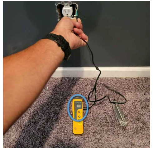
low/acceptable moisture level measured with deep wall probes
