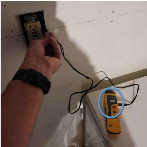
low/acceptable moisture level measured with deep wall probes
