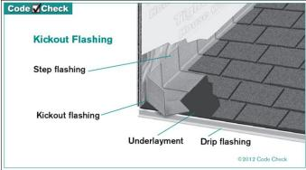
(3) Some kickout flashings were installed improperly and have the potential to allow for moisture intrusion. Have them properly re-installed.
